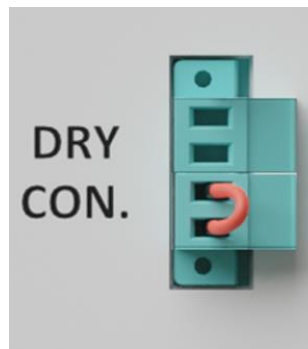
DRY CON connector with installed jumper
